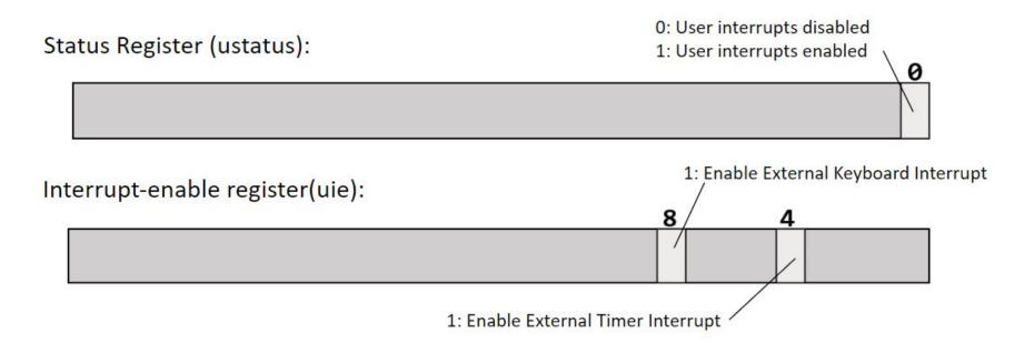
Keyboard and timer interrupts are both user interrupts. The bits above need to be set to enable keyboard and timer interrupts.
